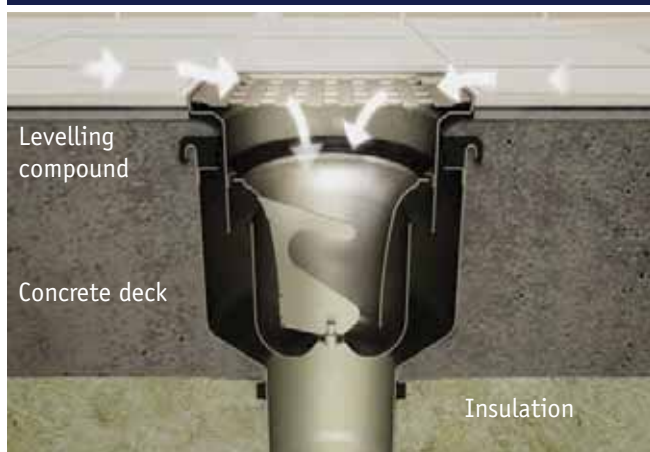
Concrete and tiles without membrane
